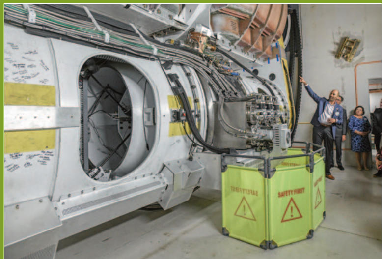
Stuart Burri, MD, chairman of Radiation Oncology at Atrium Health Levine Cancer, took attendees on a tour of the 110-ton proton accelerator unit, called the cyclotron, which powers proton beam therapy.
